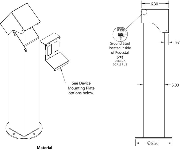
14 Ga. 304 Stainless Steel: Pedestal Body, Cover, Device Mounting Plate 7 Ga. 304 Stainless Steel: Integral Base
